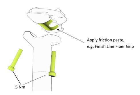
The two bolts clamping the saddle rails should be tightened evenly to 5 Nm. We recommend adding friction paste below the lower cradle. When installing the seatpost in the frame, friction paste must be applied.
