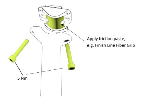
The two bolts clamping the saddle rails should be tightened evenly to 5 Nm. We recommend adding friction paste below the lower cradle. When installing the seatpost in the frame, friction paste must be applied.
