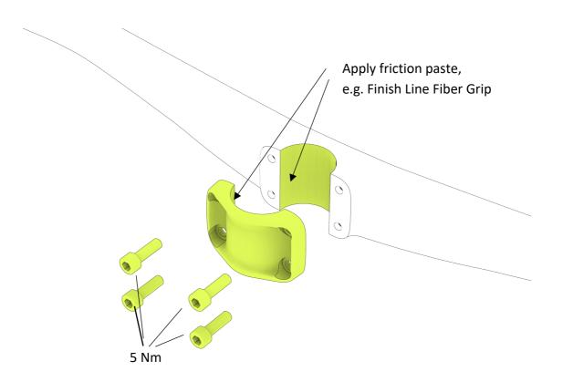
Max torque for control levers (shifting, brake, seatpost, suspension) and lock on grips is 4 Nm. The handlebar may be cut to your preferred width.
